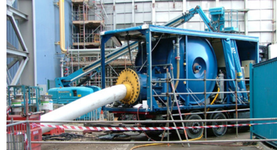
CIPP installation unit
